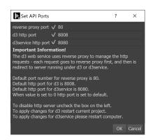
The HTTP API port settings are now configurable via d3manager under Machine Settings -> Set API Ports.
